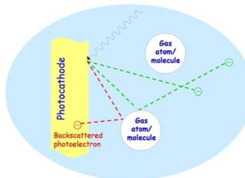
Addition of CH<sub>4</sub> or CF<sub>4</sub> to noble gases efficiently increases photoelectron transmission and drift velocity, due to the important role played by the vibrational excitation of the molecules at low electron impact energies
