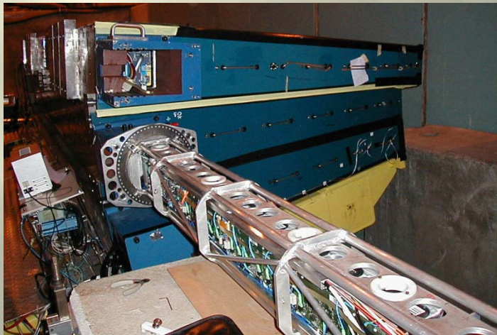
10,000 Hamamatsu R7877 Metal package Metal channel dynodes
