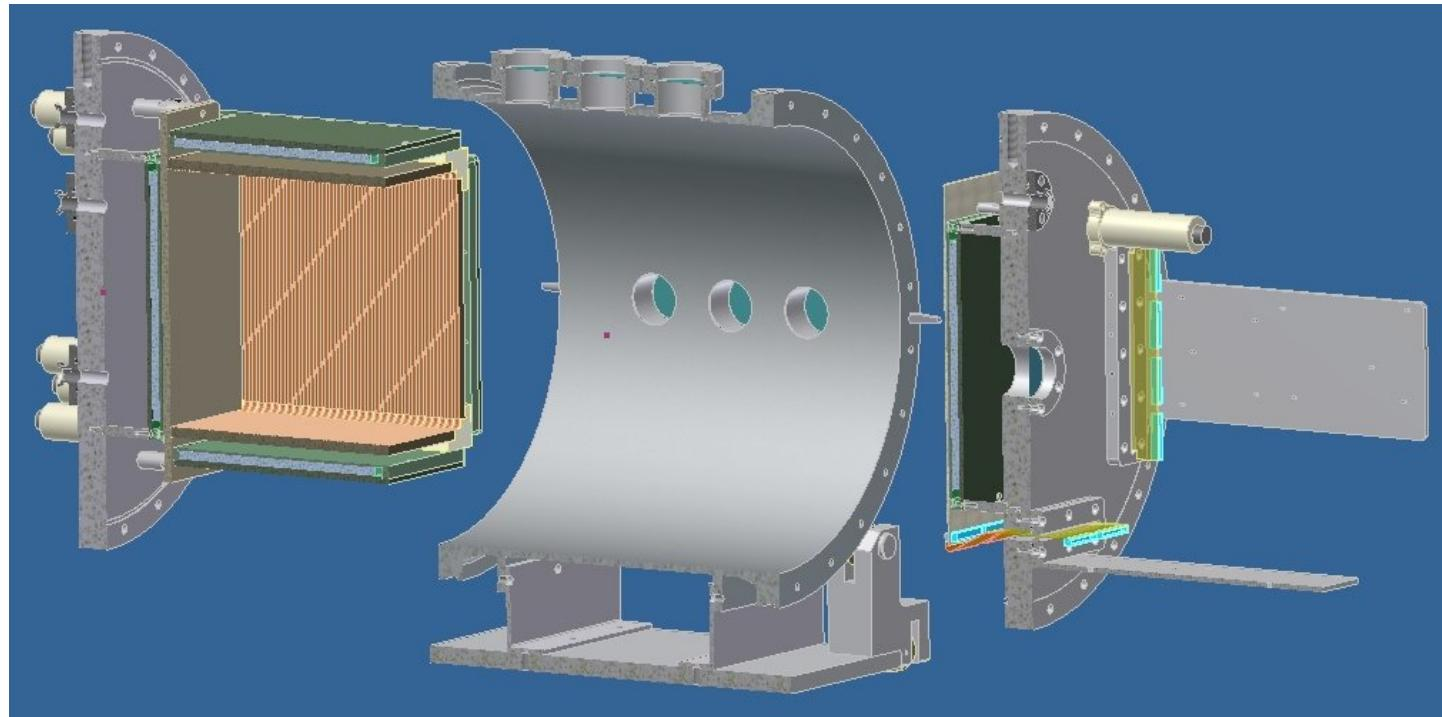
Al vessel,  $H = 500$  mm,  $\Phi = 500$  mm
