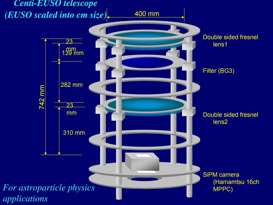
Centi-EUSO telescope with MPPC camera
