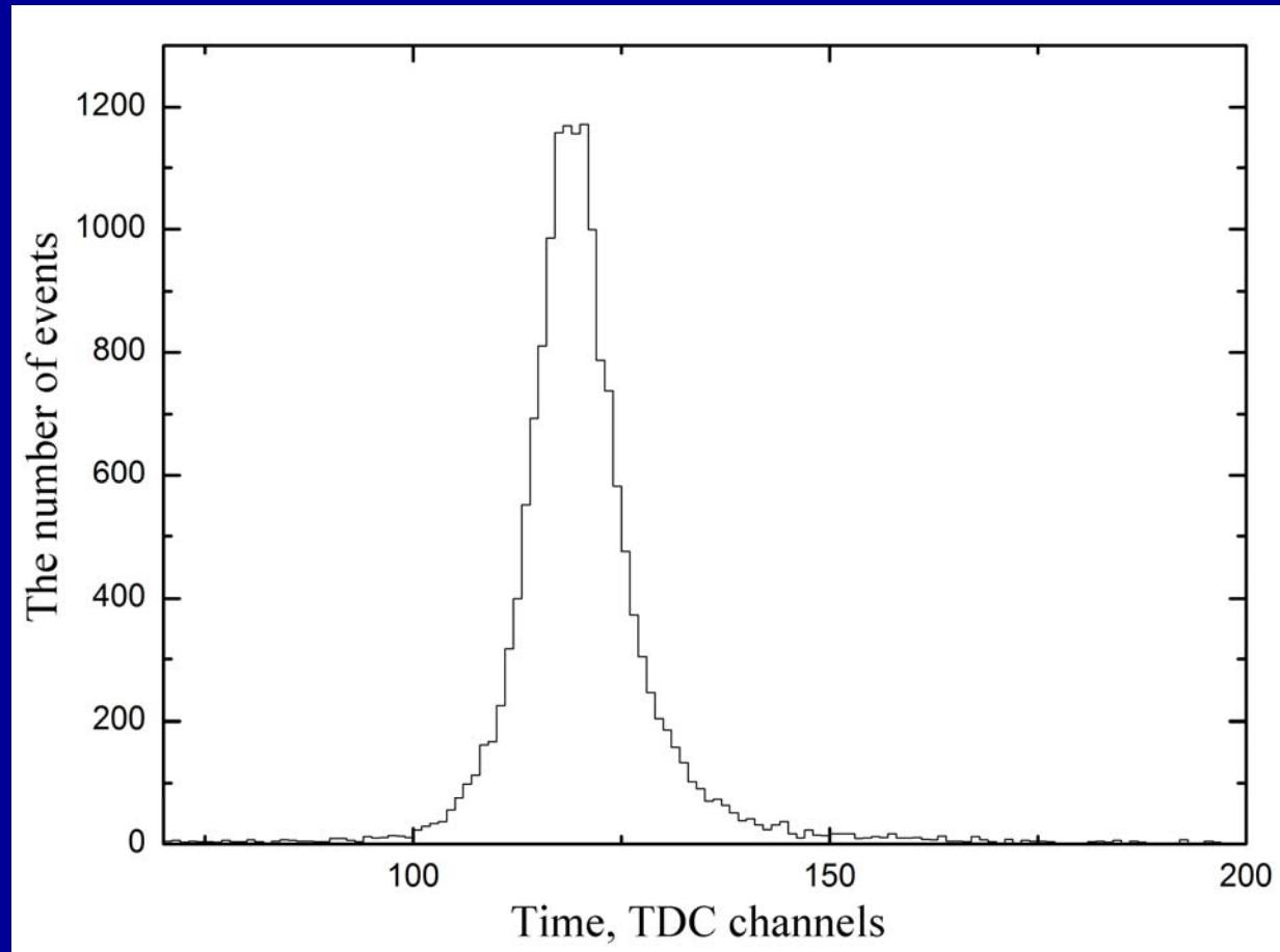
$\Delta t_{\text{hpd}} \sim 750 \text{ ps (FWHM)}$ ;  $\Delta t_{\text{LED}} \sim 700 \text{ ps}$
