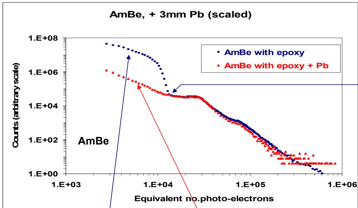
Spectra with Pb scaled to match epoxy structures (Source-APD distance larger)
