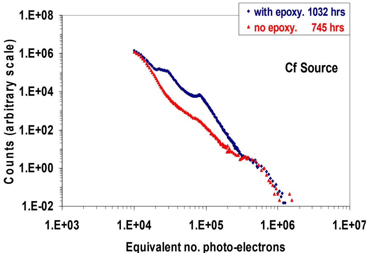
Compare to APD with epoxy removed
