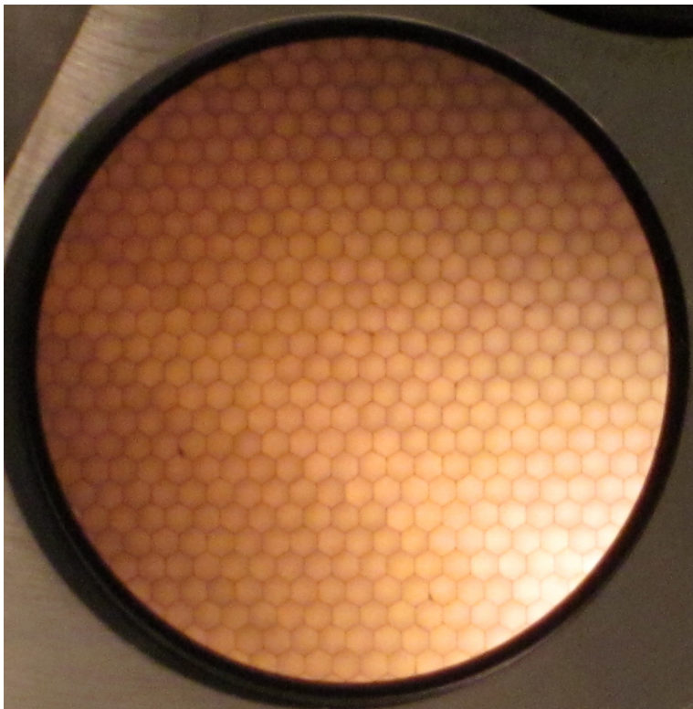
Visible light transmission for a 20 \mu\text{m} pore borosilicate microcapillary ALD MCP .
