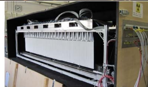
Automated source positioning: accuracy: 0.1 mm
