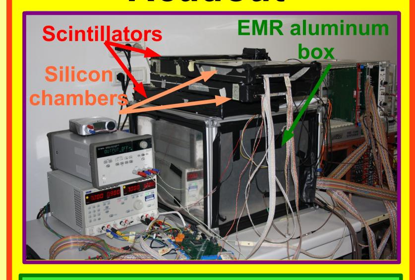
EMR aluminum the (containing the scintillator bars, the detectors and the electronics), there are two scintillators for the trigger and two silicon chambers for the particle track reconstruction. The readout for both the SiPMs and the MAPMT is performed by two 64 – channel Maroc (Multi Anode ReadOut Chip) v3 boards. Each channel features a preamplifier, a slow and a fast shaper, a discriminator and a sample & hold circuit. The Maroc3 board can be operated in an analog and a digital way.
