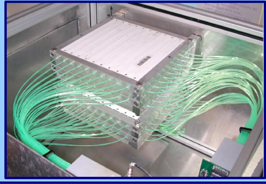
EMR (Electron Muon Ranger) Prototype Prototype of a traker for the MICE experiment composed of 8 x-y planes of plastic scintillator bars with a 1.5x1.9 cm<sup>2</sup> cross section and 19 cm long, read out by 4 0.8 mm WLS fibers. The readout of the scintillation light is performed with both SiPMs and a 64 channel multianode PMT (MAPMT, R7600-00-M64, H7546B assembly - Hamamatsu).
