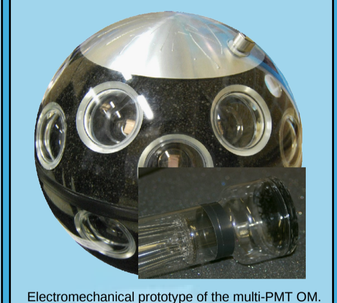
Electromechanical prototype of the multi-PMT OM. Dummy PMT from ETEL is shown in the insert
