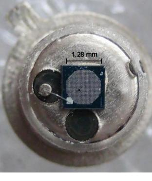
The pixels are divided by grooves, filled with an optical nontransparent material to suppress optical crosstalk between the pixels [3].
