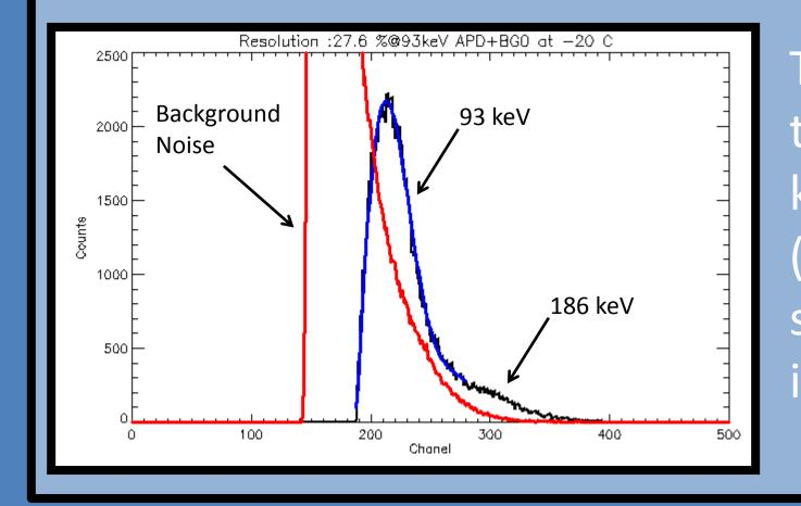
This has shown that we can obtain in the laboratory a threshold around 75 keV, close to the IXO/HXI specified ones (60 keV). More measures with different settings and temperatures will be done in the next future.
