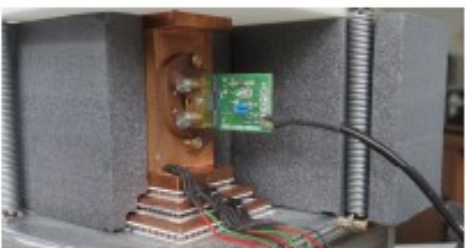
Cooling unit: 3 Peltier elements stacked on a large aluminum heat sink with forced airflow. Isolation partly opened for taking photo
