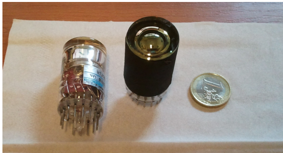
HAMAMATSU PMT (R7378A) with radiation hard fused silica incoming window
