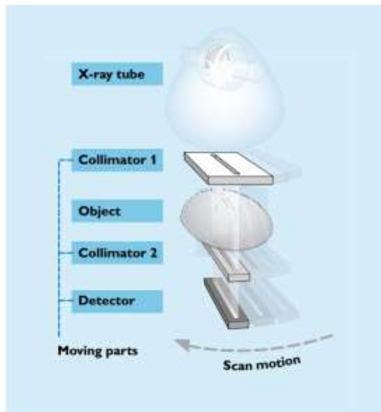
Figure 7 Multi-slit scanning technology used in Philips MicroDose.
