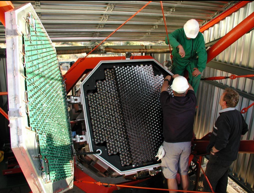
4 cameras H.E.S.S 1 800 kg, 1,5x1,6m 2 , 960 PMT
